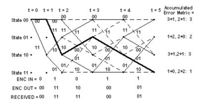
At t = 5, the path through the trellis corresponding to the actual message, shown in bold, is still associated with the smallest accumulated error metric. This is the thing that the Viterbi decoder exploits to recover the original message.
