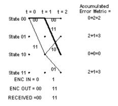
That's all the computation for t = 2. What we carry forward to t = 3 will be the accumulated error metrics for each state, and the predecessor states for each of the four states at t = 2, corresponding to the state relationships shown by the solid lines in the illustration of the trellis.
