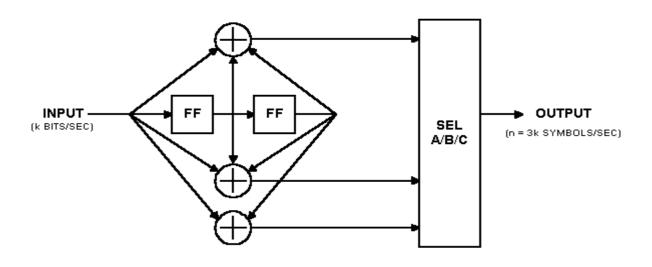
This encoder has three modulo-two adders, so for each input bit, it can produce three channel symbol outputs. Of course, with suitable puncturing patterns, you can create higher-rate codes using this encoder as well.
