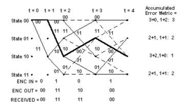
Notice that at t = 4, the path through the trellis of the actual transmitted message, shown in bold, is again associated with the smallest accumulated error metric. Let's look at t = 5:
