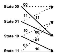
The two-bit numbers labeling the lines are the corresponding convolutional encoder channel symbol outputs. Remember that dotted lines represent cases where the encoder input is a zero, and solid lines represent cases where the encoder input is a one. (In the figure above, the two-bit binary numbers labeling dotted lines are on the left, and the two-bit binary numbers labeling solid lines are on the right.)
