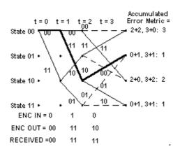
Note that the third channel symbol pair we received had a one-symbol error. The smallest accumulated error metric is a one, and there are two of these.
